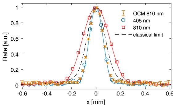
**Fig. 4.** Projection of the PSF of low-NA single-lens imaging at different light sources. Measurements with coherent light at 810 nm (squares) and 405 nm (circles) are shown with their theoretical curves. The biphoton OCM PSF at 810 nm (dots) closely agrees with 405 nm and confirms its doubled resolution. Statistical  $2\sigma$  errors are shown. The OCM PSF surpasses a theoretical SQL-scaling PSF of the centroid of two classically correlated photons at 810 nm (dashed line).
