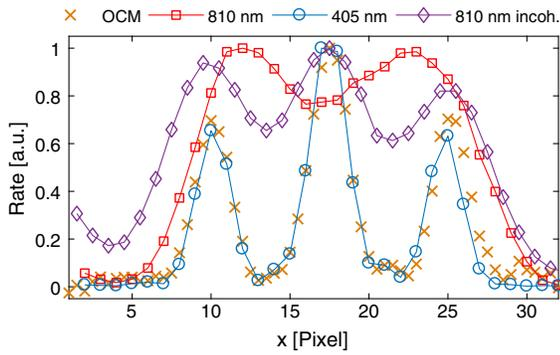
**Fig. 3.** Triple-slit object of 70  $\mu\text{m}$  linewidth is used for resolution comparison. Cross sections in low-NA imaging using biphoton OCM at 810 nm (crosses), spatially coherent illumination at 810 nm (squares) and 405 nm (circles), and incoherent light at 810 nm (diamonds) are shown. OCM shows an advantage that is practically identical to the double resolution given with 405 nm.
